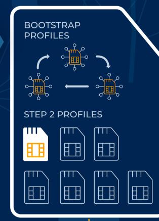
Preloaded with multiple profiles (called bootstraps) and can push more profiles over-the-air should a better network become available.
